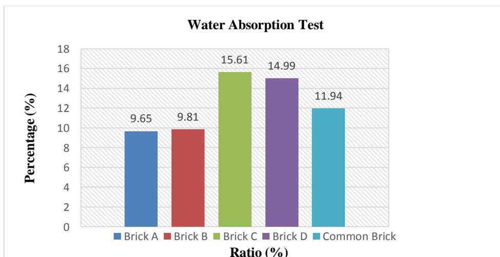
Figure 3: Water Absorption Test (%)
