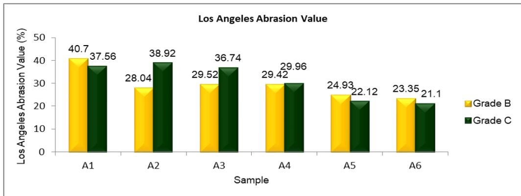
Figure 2: Result of LA Abrasion Value
