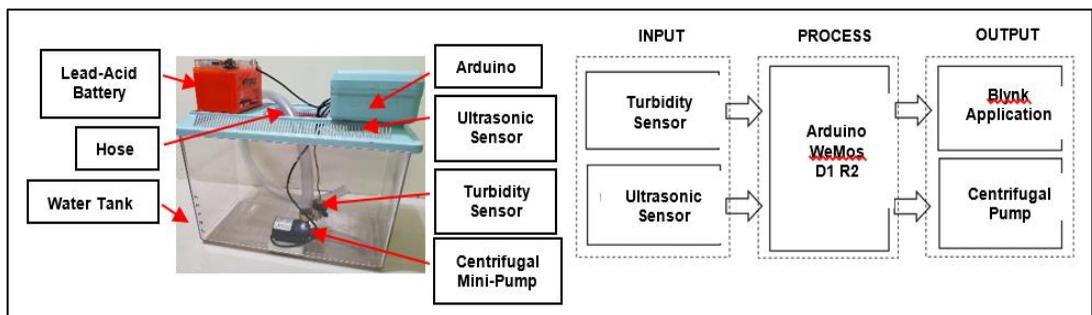
Figure 2: Autonomous Grease Trap Maintenance System and Block Diagram of the System
