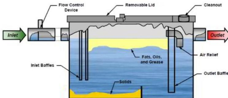
Figure 1: Hydromechanical Grease Interceptor (Hall's Septic Services Inc., 2021)
