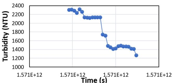
Figure 6: Relationship between water turbidity and operating time
