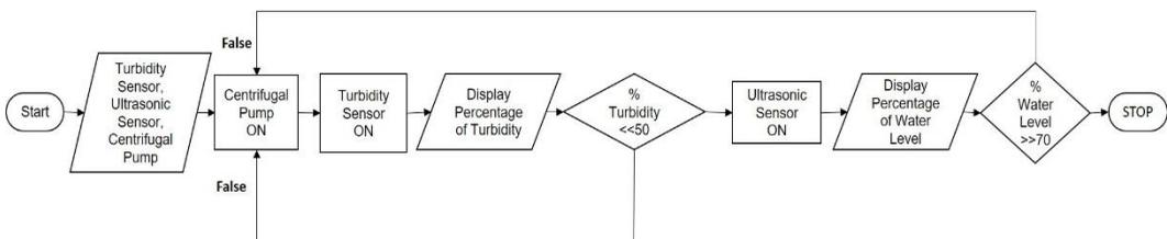
Figure 3: Flowchart of software design
