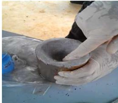
Figure 1: Preparation of Emulex Shaped Charge.
