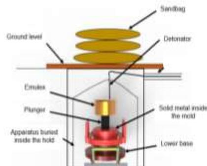
Figure 2: Schematic Diagram of Underground Explosion Pressing
