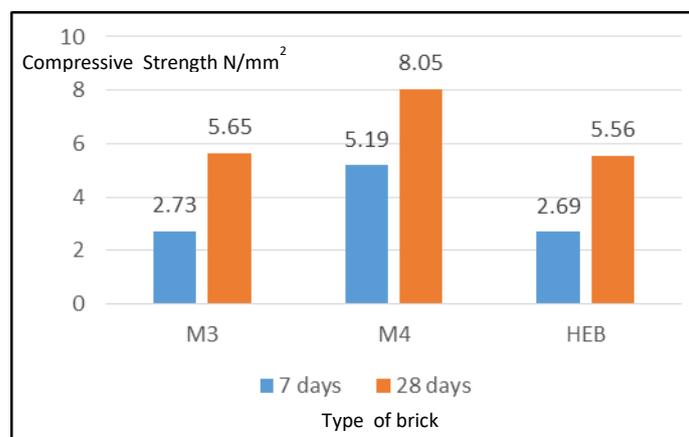
Figure 2: Compressive strength result
