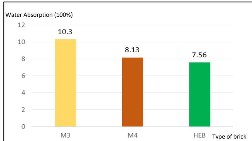
Figure 4: Water absorption result
