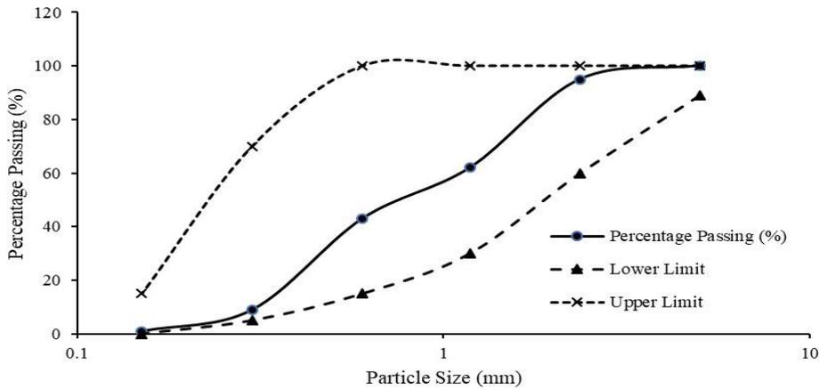
Figure 2: Grading Curves of Sand
