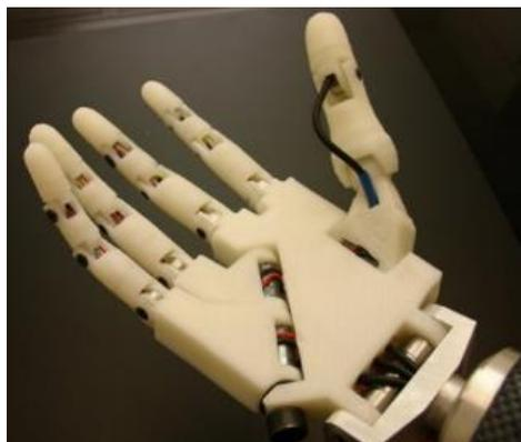
Figure 2: Inmoov Robotic hand design (Langevin, 2012).
