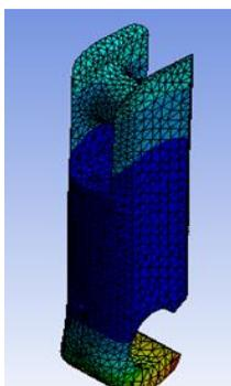
Maximum deformation at the C-section
