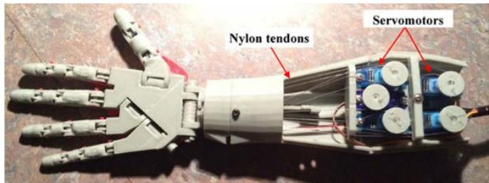
Figure 1: Inmoov open source 3D printed Prosthetic arm. (Langevin, 2012)
