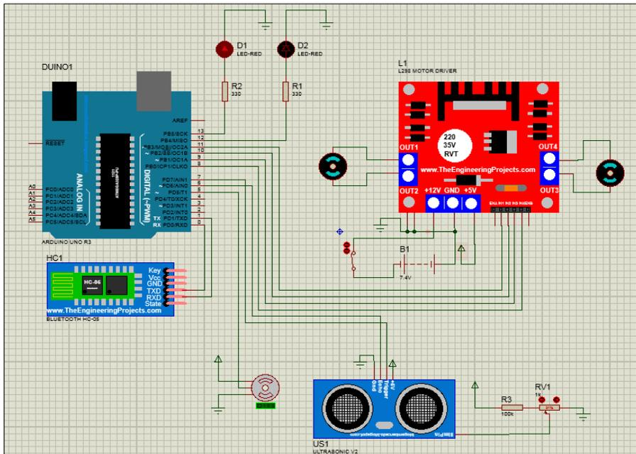
Figure 2: Schematic Diagram of Marine Robot
