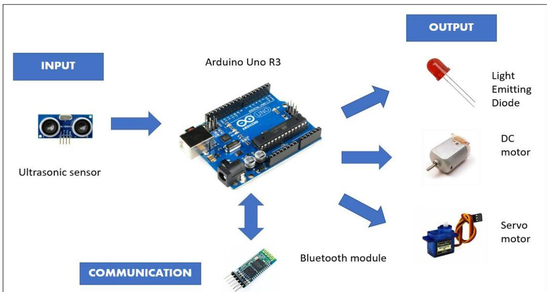
Figure 1: Block Diagram of Marine Robot
