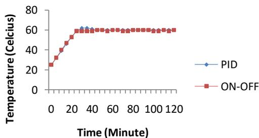
Fig. 2 *PID and On-Off Controller test results***c. Temperature Accuracy Testing**
