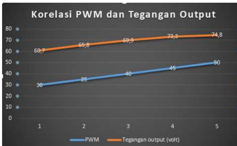
Fig 3. PWM and Output Voltage
