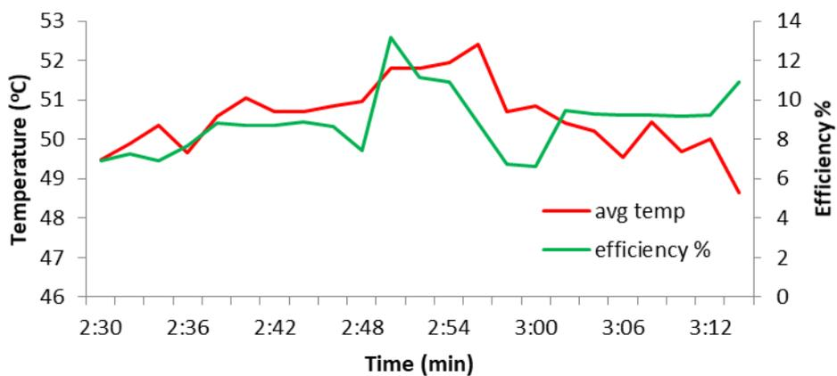
Fig.4: Average temperature and PV efficiency vs time (unfiltered)
