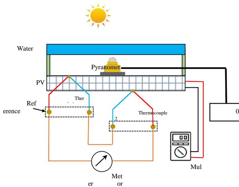
Fig.1: The schematic of an experiment setup for a 10mm filtered PV panel with water
