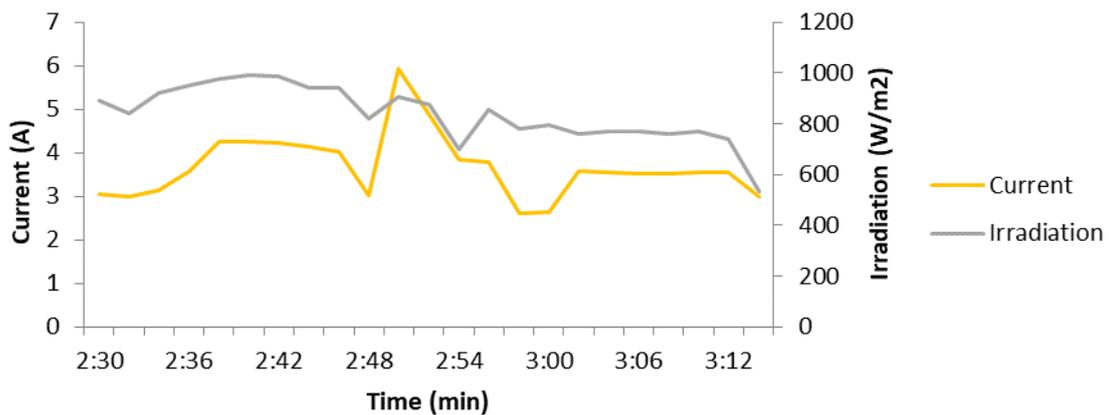
Fig.3: Transmitted irradiation and current vs time (unfiltered)
