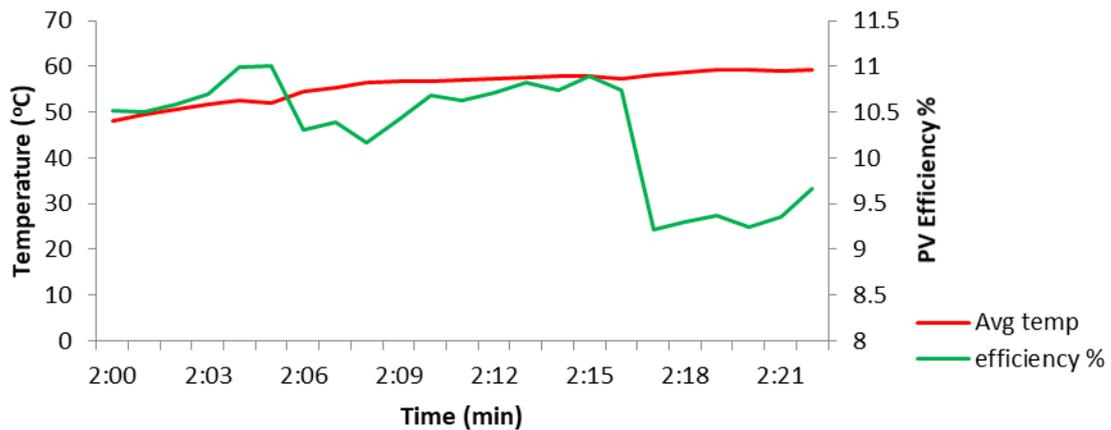
Fig.7: Average temperature and PV efficiency vs time (10mm filtered PV with water)
