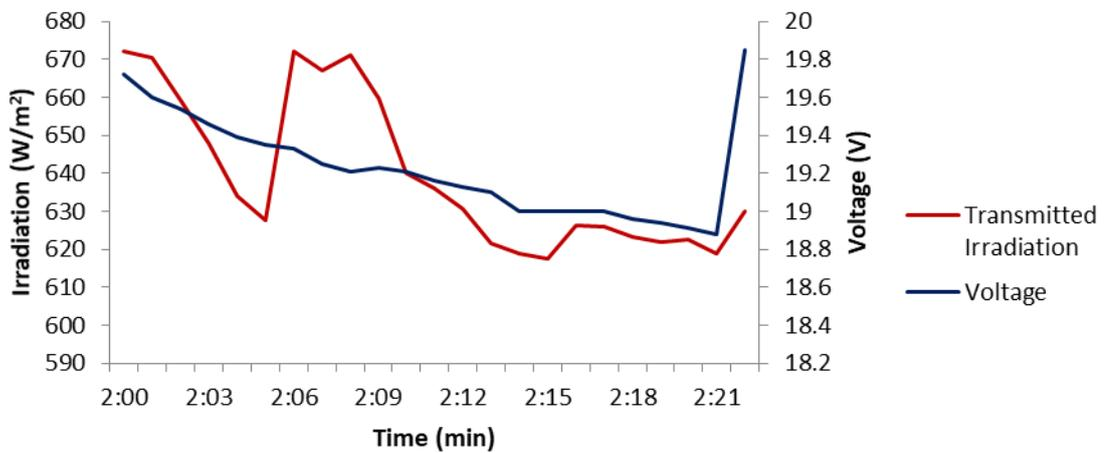
Fig.5: Transmitted irradiation and voltage vs time (10mm filtered PV with water)
