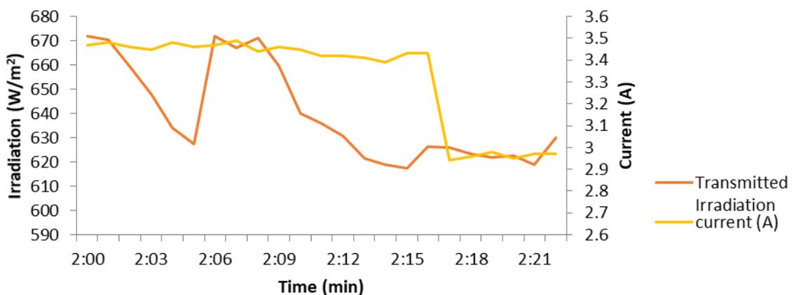
Fig.6: Transmitted irradiation and current vs time (10mm filtered PV with water)
