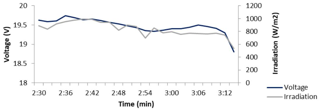
Fig.2: Transmitted irradiation and voltage vs time (unfiltered)
