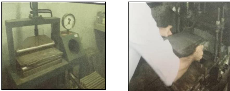
Figure 3: Transverse Strength Mechine used Terreal-Vitage Tile Sdn. Bhd
