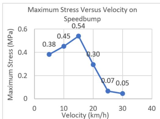
Figure 8: Graph of maximum stress versus velocity on speedbump
