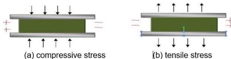
Figure 1: Two different types of stress on piezoelectric to generate piezo electricity
