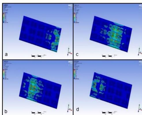
Figure 7: (a) initial (b) second (c) third (d) final stress on PZT Tile at 15km/h
