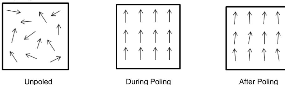
Figure 2: Electric dipoles of piezoelectric material. (Kok, 2010)
