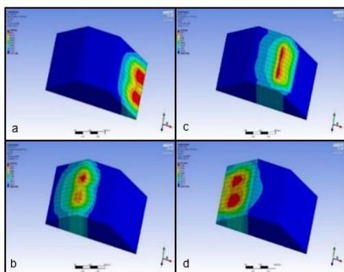
Figure 6: (a) initial (b) second (c) third (d) final stress on speedbump at 15km/h
