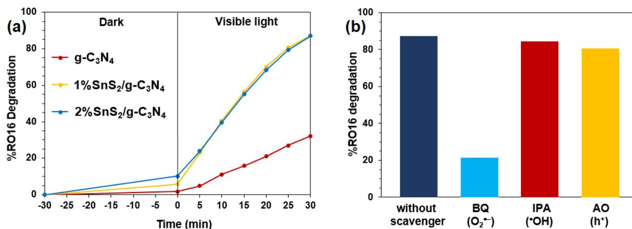
Figure 3: Photocatalytic degradation of RO16 (a) and the presence of different scavengers over the photocatalytic activity of 1%SnS<sub>2</sub>/g-C<sub>3</sub>N<sub>4</sub> (b)
