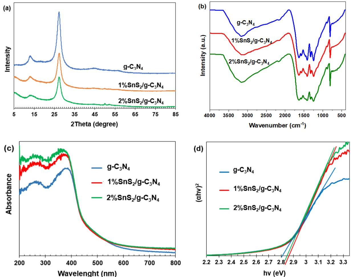
Figure 1: XRD patterns (a), FTIR spectra (b), DRS spectra (c) and Talc plots of synthesized photocatalysts (d)
