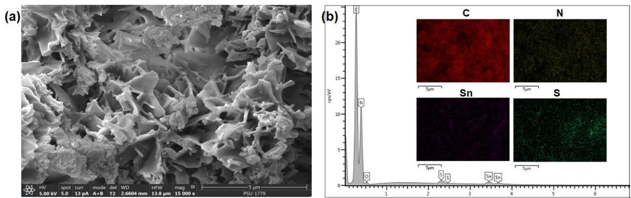
Figure 2: SEM-EDS mapping of 1%SnS<sub>2</sub>/g-C<sub>3</sub>N<sub>4</sub> photocatalyst
