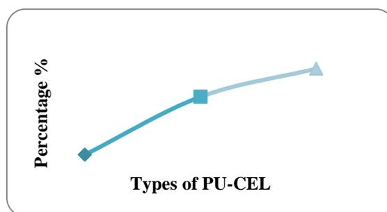
Fig. 5: Graph showing the increasing trend of weight loss in percentage value for PU-CEL 0, PU-CEL 20 and PU-CEL 40 after 30 days.
