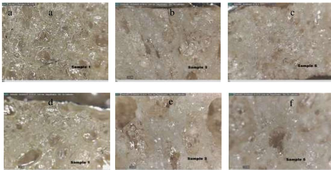
Fig. 6 Magnification of PU-CEL at 20x (a: PU-CEL 0, b: PU-CEL 20, c: PU-CEL 40); Magnification of PU-CEL at 50x (d: PU-CEL 0, e: PU-CEL 20, f: PU-CEL 40)
