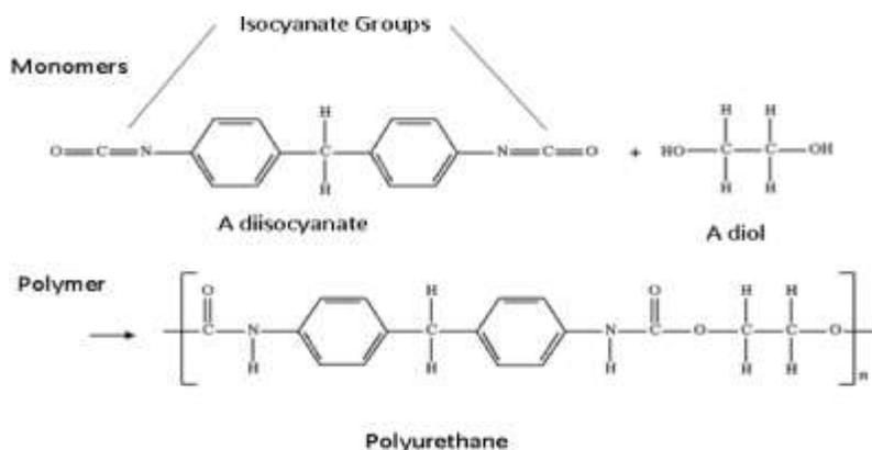
Fig. 1: Structure of monomers and polymers of polyurethane
